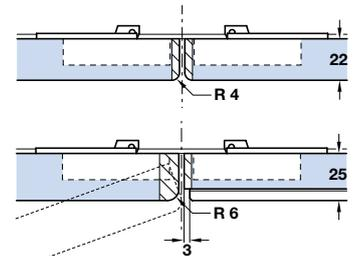
For door thickness 20+ mm, edges must be radiused
