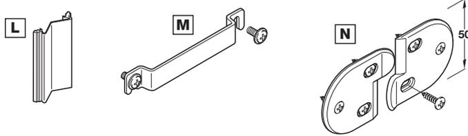
**Note:** When all door panels are opened and pushed to one side, there is the danger of the cabinet tipping over, to prevent this use this safety fitting to anchor the unit to a back wall
