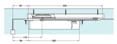
Fixing position: Where intumescents are to be fitted, 1 mm must be added to all dimensions (see fitting instructions)
