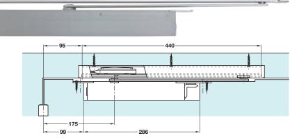
Fixing position: With intumescents fitted, 1 mm must be added to all dimensions (see fitting instructions)
