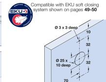
Drilling diagram for F
