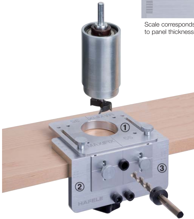
Drilling position for connector housings (drilling dimension B = 55 mm)
