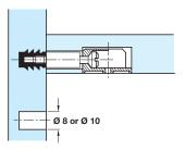
Connecting bolt with M6 thread for use in dowel or sleeve for push-fit or press-fit fastening in Ø 8 or Ø 10 mm hole
