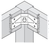
Leg screw fixed through centre hole of corner brace
