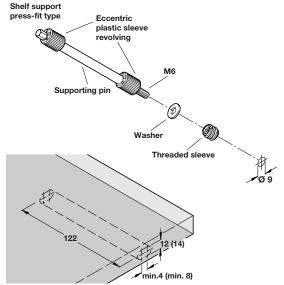
Dimensions in brackets are for shelf thickness 22 mm using 14 mm size shelf support
