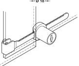
For infront glass sliding doors: Rack is clamped on to the rear glass panel. Clip on lock and allow to engage in the rack. In order to unlock, remove the lock from the rack and put aside.
