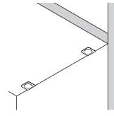
1. Push connector into drill hole
