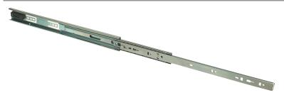
For optimum performance allow between +0.2mm and +0.5mm over the nominal runner thickness, for the runner space.
