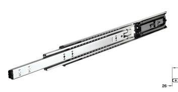
Side spaceFor optimum performance allow between +0.2mm and +0.5mm over the nominal runner thickness, for the runner space.
