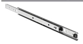
For optimum performance allow between +0.2mm and +0.5mm over the nominal runner thickness, for the runner space.
