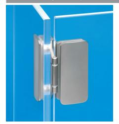
> For glass thickness (side wall and door panel): 5-8 mm > Opening angle 180° > Axle Ø 5 mm, length 32 mm
