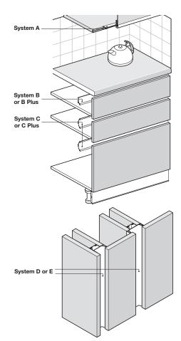
GOLA System A profile, for horizontal fixing under wall units, without soft lip shock absorber
