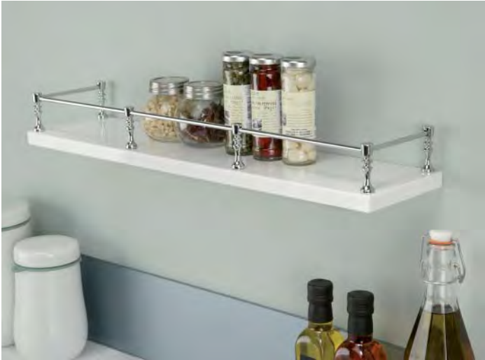
Posts press fit into Ø 6 mm, 12.5 mm deep holes
