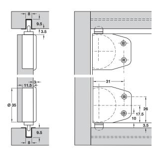
> Important: All the weight of both doors in any folding pair is supported entirely by the hinges
