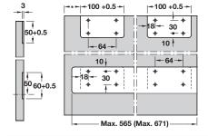
Recesses for cabinet side panel for screw on/retaining plates
