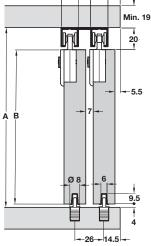
With screw fixing tracks B = A - 24 mm
