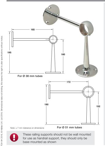
These railing supports should not be wall mounted for use as handrail support, they should only be base mounted as shown
