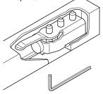
The retaining force can be adjusted with an allen key
