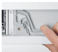
Position it flush with the front panel and screw to the drawer bottom panel
