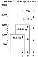
Sample measurements for 20 mm thick wood Hinge distance min. 500 mm Door width up to 600 mm The door's width must not exceed its height
