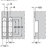
With wood thickness 18 mm: A = 9 mm With wood thickness min. 20 mm: A = 10 mm
