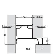
> For fixing between the cabinet and door
