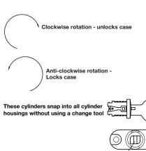
To install: Line up lock so that key lines up with notch in cylinder housing as shown
