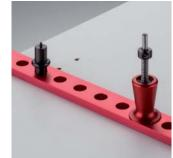
The drilling jig is moved and fixed wth the locating pin for longer rows of series
