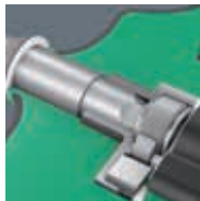
Ratchet mechanism in the handle
