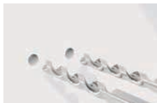
Drill Ø 8 mm hole for connecting bolt
