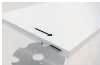
Mill lengthways groove for connector
