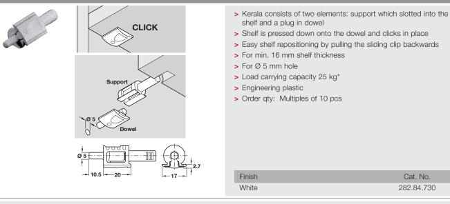
\*Load carrying capacity applies to 4 shelf supports bearing an evenly distributed load. Testing was carried out according to DIN EN 14749: 2005, clause 6.3.3 "Strength of shelf supports"
