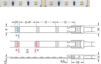
Cut LED strip light to length (one contact side remains on the remainder piece; reusable)
