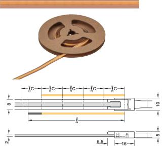
Yellow: illuminated strip section Grey: non-illuminated strip section (when cut between 2 cutting marks) C = Section length
