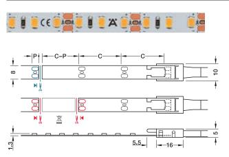
Cut LED strip light to length (one contact side remains on the remainder piece; reusable)
