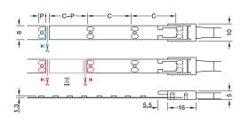
Cut LED strip light to length (one contact side remains on the remainder piece; reusable)
