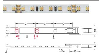
Cut LED strip light to length (one contact side remains on the remainder piece; reusable)
