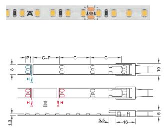
Cut LED strip light to length (one contact side remains on the remainder piece; reusable)
